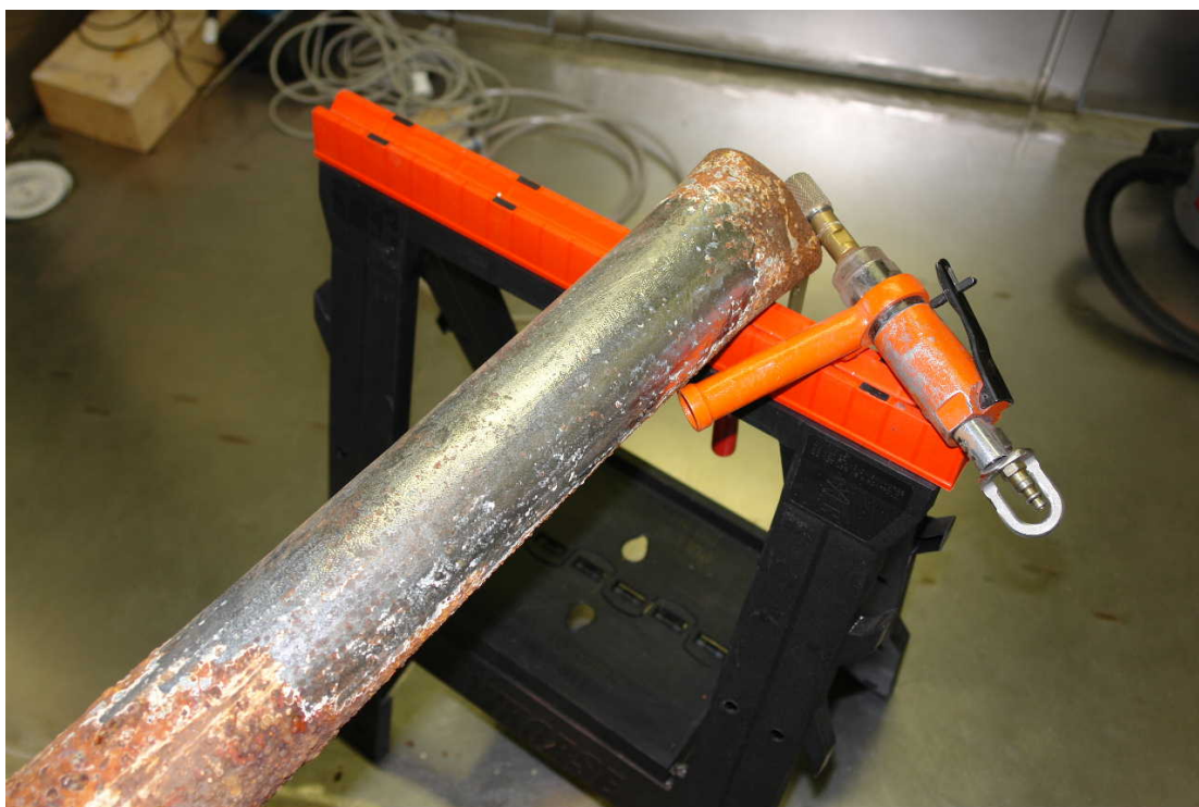
Figure 4. Metal part 3: 3½ inch pipe. The wall thickness is 5.5 mm.
