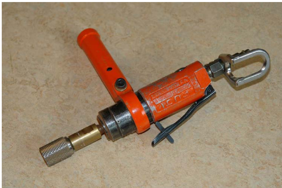
Figure 1. Cold grinding tool with rotating file. File diameter: 25 mm, width: 30 mm.
