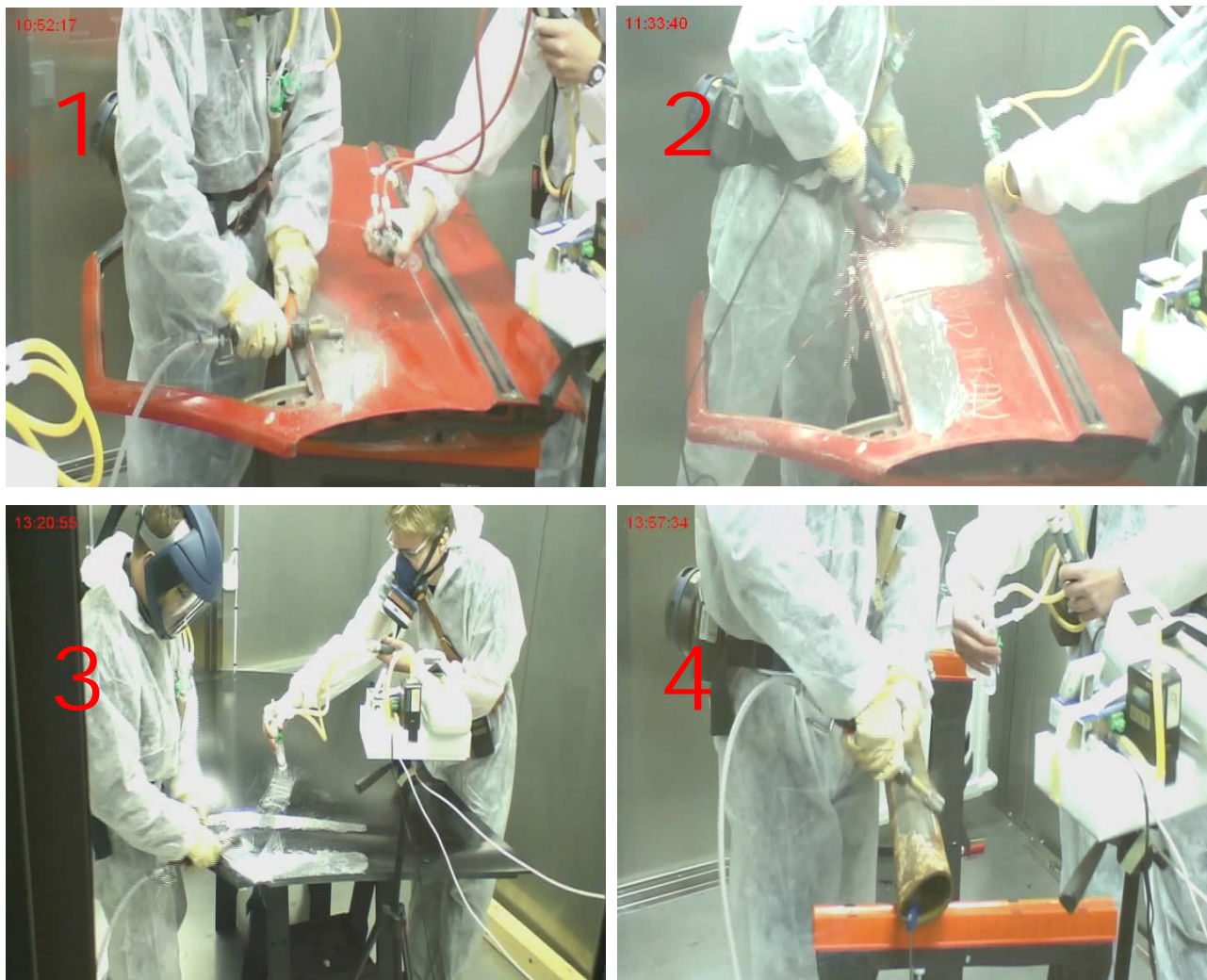
Figure 6. Pictures showing (1) rotating file on car door, (2) angle grinder on car door, (3) rotating file on car bonnet and (4) rotating file on 3½ inch pipe.
