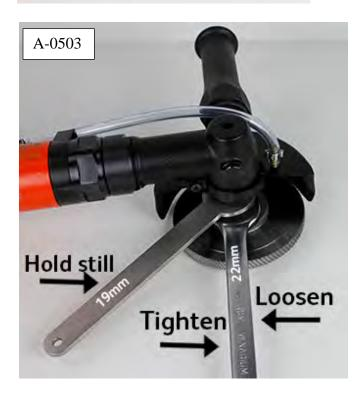
When attaching and removing the Weld Seam Disk (A-0503) to the A-0105 Air Tool you will need the following accessories:
