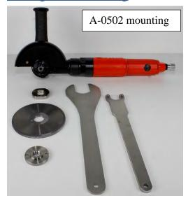
When attaching and removing the Cutting Disk (A-0502) to the A-0105 Ex Air Tool you will need the following accessories:
