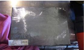
005 Test plate 1 profile 2 mils, right angle grinder
