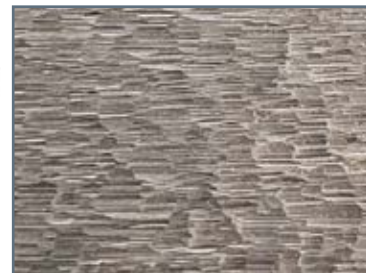
A-0002 Surface. Average 43 \mu\text{m}
