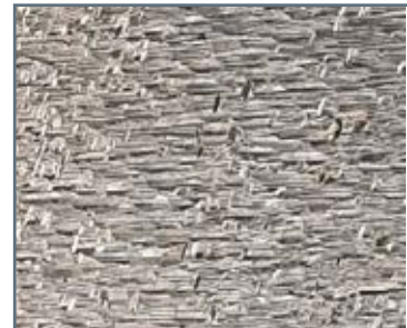
A-0001 Surface. Average 76 \mu\text{m}
