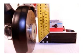
Make sure the cutting disc is attached with a 90deg angle to the surface.
