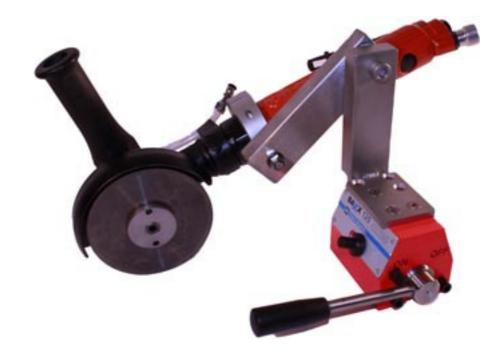
To setup the Pendulum arm, insert the A-0105 (Fuju angle grinder) into the "machine locking" and use an Allan key to fasten the two fastening screws. Make sure the machine is fastened properly.
